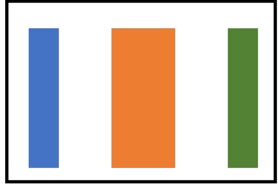
Fig. 3: An approximation of our depth calculation strategy. The entire picture represents the depth image exported by [23]. The left depth is extracted as an average over the blue region, the right over the green region, and the center over the orange region.
